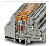
Knife disconnect terminal block, With test socket screws for insertion of test plugs, Connection type: Screw connection, Cross section: 0.2 mm² - 4 mm², AWG: 24 - 12, Nominal current: 10 A, Nominal voltage: 400 V, Length: 106 mm, Width: 6.2 mm, Color: gray, Assembly: NS 35/7,5, NS 35/15, NS 32
