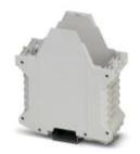
Component housing without vents, Lower part, Cross connection: DIN rail bus connector, Color: light gray, Width: 45 mm, Constructional height: 114.5 mm, Number of positions cross connector: 5
