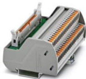
VARIOFACE interface module for Siemens SIMATIC® S7-300, with SIMATIC®-specific labeling (1 - 40), with push-in connection, module width: 107.9 mm
