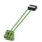
Cable set for signal transmission on the termination carrier for safety relay modules from the PSR-FSP series. Connection of terminal points A1 and A2 (signal transmission) with screw connection to the signal PCB via a 6-pos. PTSM connector.
