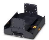
Installation component housing with vents, Lower part, Cross connection: DIN rail bus connector, Color: black, Width: 53.6 mm, Constructional height: 49 mm, Number of positions cross connector: 16
