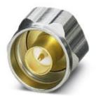
A termination resistor must be screwed on at the end of the leaky wave conductor which does not contain any wireless part. It guarantees an antenna cable termination with the correct impedance and is important for every wireless installation.
