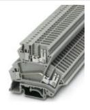
Feed-through terminal block, Connection type: Screw connection, Slip-on connection, Cross section: 0.2 mm<sup>2</sup> - 4 mm<sup>2</sup>, AWG :24- 12, Width: 6.2 mm, Color: gray, Mounting: NS 35/7,5, NS 35/15, NS 32
