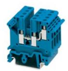
1-level terminal block with double connection on one side, cross section: 0.2 - 4 mm², AWG: 24 - 12, width: 6.2 mm, color: blue
