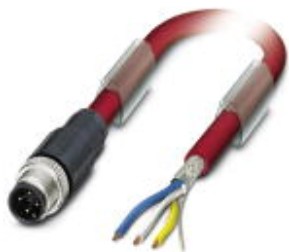
Bus system cable, CC link (10 Mbps), 4-position, PVC, red, shielded, Plug straight M12, A-coded, on free cable end, Cable length: 15 m
