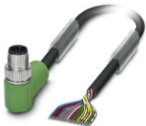
Sensor/Actuator cable, 17-position, PVC, black RAL 9005, Plug angled M12 SPEEDCON, A-coded, on free cable end, Cable length: 3 m
