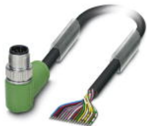
Sensor/Actuator cable, 17-position, PVC, black RAL 9005, Plug angled M12 SPEEDCON, A-coded, on free cable end, Cable length: 1.5 m
