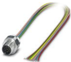
Sensor/actuator flush-type plug, 8-pos., M12, front/screw mounting with Pg9 thread, can be positioned, with 0.5 m TPE litz wire, 8 x 0.25 mm 2 , high-grade steel version
