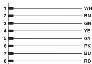
Contact assignment of the M12 plug and the M12 socket
