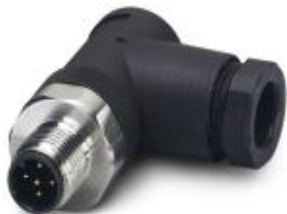
Sensor/actuator connector, male, angled, 5-pos., M12, screw connection, high-grade steel knurl, cable screw connection Pg9
