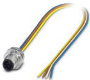
Bus system flat-type plug, PROFINET, 4-position, PlugLink:straightLink:M12-SPEEDCON, D-coded, Front mounting, M16 x 1.5, Individual wires, Cable length: 0.5 m
