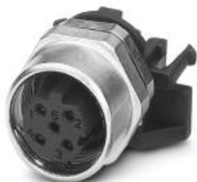
Bus system flush-type socket, Ethernet, 4-pos., M12 SPEEDCON, D-coded, rear/screw mounting with M12 thread, with polarity protection, with straight solder connection
