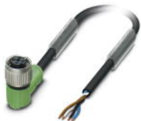
Sensor/Actuator cable, 4-position, PUR halogen-free, black-gray RAL 7021, free cable end, on Socket angled M12 SPEEDCON, A-coded, Cable length: 1.5 m
