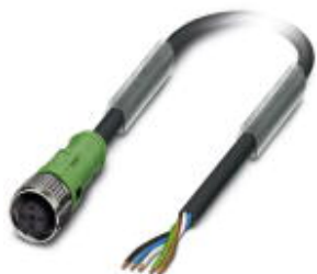
Sensor/Actuator cable, 5-position, PUR halogen-free, black-gray RAL 7021, free cable end, on Socket straight M12 SPEEDCON, A-coded, Cable length: 5 m
