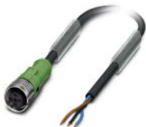
Sensor/Actuator cable, 3-position, PUR halogen-free, black-gray RAL 7021, free cable end, on Socket straight M12 SPEEDCON, A-coded, Cable length: 10 m
