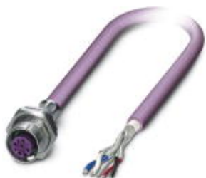
Bus system flush-type socket, DeviceNet/CANopen, 5-pos., M12, shielded, A-coded, rear/screw mounting with M16 thread, with 1 m bus cable, 2 x 0.2 mm 2 , 2 x 0.32 mm 2
