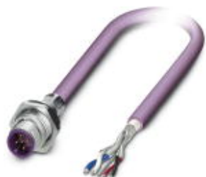
Bus system flush-type plug, DeviceNet/CANopen, 5-pos., M12, shielded, A-coded, rear/screw mounting with M16 thread, with 0.5 m bus cable, 2 x 0.2 mm 2 , 2 x 0.32 mm 2
