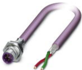
Bus system flush-type plug, PROFIBUS, 2-pos., M12, shielded, B-coded, rear/screw mounting with M16 thread, with 5 m bus cable, 2 x 0.25 mm 2
