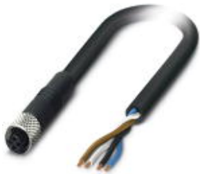
Sensor/Actuator cable, 4-position, PUR, black RAL 9005, free cable end, on Socket straight M5, A-coded, Cable length: 5 m
