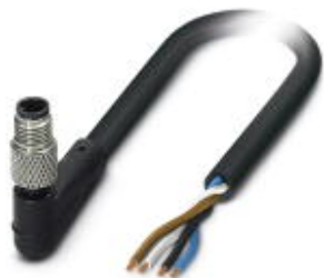
Sensor/Actuator cable, 4-position, PUR, black RAL 9005, Plug angled M5, A-coded, on free cable end, Cable length: 3 m
