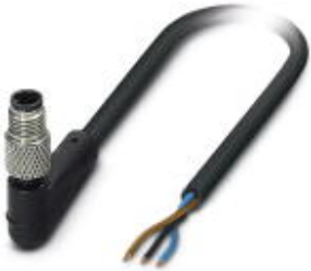
Sensor/Actuator cable, 3-position, PUR, black RAL 9005, Plug angled M5, A-coded, on free cable end, Cable length: 1.5 m
