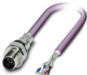
Bus system flush-type plug, DeviceNet/CANopen, 5-pos., M12, shielded, A-coded, front/screw mounting with M16 thread, with 5 m bus cable, 2 x 0.2 mm 2 , 2 x 0.32 mm 2
