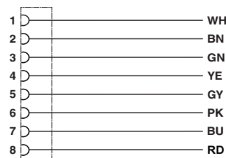
Contact assignment of the M12 socket
