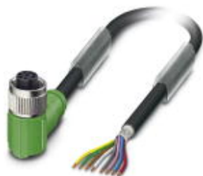
Sensor/Actuator cable, 8-position, PUR halogen-free, black-gray RAL 7021, shielded, free cable end, on Socket angled M12, A-coded, Cable length: 3 m
