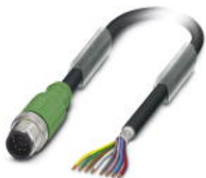
Sensor/Actuator cable, 8-position, PUR halogen-free, black-gray RAL 7021, shielded, Plug straight M12, A-coded, on free cable end, Cable length: 3 m
