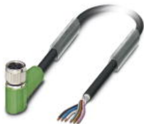
Sensor/Actuator cable, 6-position, PUR halogen-free, black-gray RAL 7021, shielded, free cable end, on Socket angled M8, Cable length: 5 m
