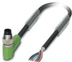
Sensor/Actuator cable, 6-position, PUR halogen-free, black-gray RAL 7021, shielded, Plug angled M8, on free cable end, Cable length: 1.5 m, Customer version
