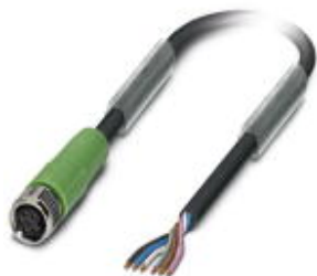
Sensor/Actuator cable, 6-position, PUR halogen-free, black-gray RAL 7021, free cable end, on Socket straight M8, Cable length: 3 m
