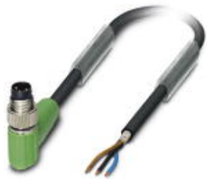
Sensor/Actuator cable, 3-position, PUR halogen-free, black-gray RAL 7021, shielded, Plug angled M8, on free cable end, Cable length: 10 m
