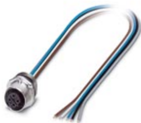
Fieldbus flush-type socket, INTERBUS/PROFIBUS, 5-pos., M12 SPEEDCON, B-coded, front/screw mounting with M16 thread, with 0.5 m TPE litz wire, 5x 0.34 mm 2
