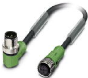
Sensor/Actuator cable, 5-position, PUR halogen-free, black-gray RAL 7021, Plug angled M12 SPEEDCON, A-coded, on Socket straight M12 SPEEDCON, A-coded, Cable length: 1.5 m
