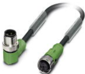
Sensor/Actuator cable, 4-position, PUR halogen-free, black-gray RAL 7021, Plug angled M12 SPEEDCON, A-coded, on Socket straight M12 SPEEDCON, A-coded, Cable length: 3 m
