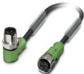
Sensor/Actuator cable, 3-position, PUR halogen-free, black-gray RAL 7021, Plug angled M12 SPEEDCON, A-coded, on Socket straight M12 SPEEDCON, A-coded, Cable length: 0.6 m
