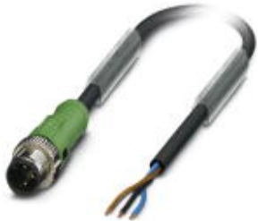
Sensor/Actuator cable, 3-position, PUR halogen-free, black-gray RAL 7021, Plug straight M12 SPEEDCON, A-coded, on free cable end, Cable length: 3 m
