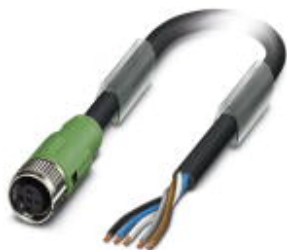
Sensor/Actuator cable, 5-position, PUR, black-gray RAL 7021, free cable end, on Socket straight M12 SPEEDCON, A-coded, Cable length: 10 m
