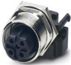
Sensor/Actuator flush-type socket, 5-pos., M12, B-coded, rear/screw mounting with M12 thread, with straight solder connection
