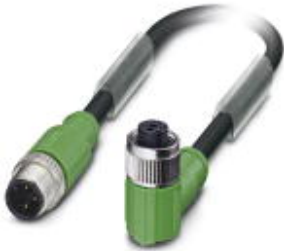
Sensor/Actuator cable, 3-position, PUR halogen-free, black-gray RAL 7021, shielded, Plug straight M12, A-coded, on Socket angled M12, A-coded, Cable length: 0.3 m
