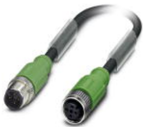
Sensor/Actuator cable, 4-position, PUR halogen-free, black-gray RAL 7021, shielded, Plug straight M12, A-coded, on Socket straight M12, A-coded, Cable length: 0.3 m
