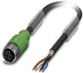
Sensor/Actuator cable, 4-position, PUR halogen-free, black-gray RAL 7021, shielded, free cable end, on Socket straight M12, A-coded, Cable length: 10 m
