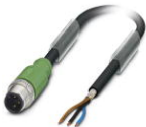
Sensor/Actuator cable, 3-position, PUR halogen-free, black-gray RAL 7021, shielded, Plug straight M12, A-coded, on free cable end, Cable length: 10 m
