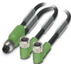
Sensor/Actuator cable, 3-position, PUR halogen-free, black-gray RAL 7021, Plug straight M8, on Socket angled M8 and Socket angled M8, Cable length: 1.5 m
