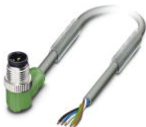
Sensor/Actuator cable, 5-position, PUR halogen-free, welding sputter-resistant, highly flexible, gray RAL 7001, Plug angled M12, A-coded, on free cable end, Cable length: 10 m, for robots and drag chains
