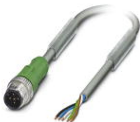
Sensor/Actuator cable, 5-position, PUR halogen-free, welding sputter-resistant, highly flexible, gray RAL 7001, Plug straight M12, A-coded, on free cable end, Cable length: 3 m, for robots and drag chains
