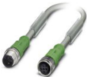
Sensor/Actuator cable, 3-position, PUR, gray RAL 7001, Plug straight M12, A-coded, on Socket straight M12, A-coded, Cable length: 3 m, for robots and drag chains
