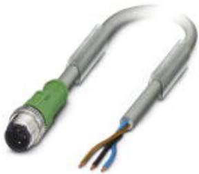
Sensor/Actuator cable, 3-position, PUR halogen-free, welding sputter-resistant, highly flexible, gray RAL 7001, Plug straight M12, A-coded, on free cable end, Cable length: 3 m, for robots and drag chains
