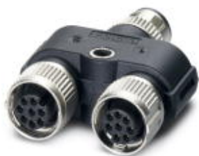
Y distributor, 8-position, shielded, Plug straight M12 SPEEDCON, A-coded, on Socket straight M12 SPEEDCON, A-coded and Socket straight M12 SPEEDCON, A-coded, Parallel distributor
