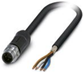
Sensor/Actuator cable, 4-position, PE-X/PE-X halogen-free, black-gray RAL 7021, shielded, Plug straight M12, A-coded, on free cable end, Cable length: 10 m, for outdoor applications, With high-grade steel knurl
